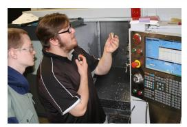
Students gain a global understanding of precision machining, the process of removing metal to create extremely accurate parts. They learn all aspects of the advanced manufacturing industry, including how to operate CNC (Computer Numerical Controlled) lathes, mills and power saws. The creation of blueprints and designs using industry-driven software and technology is covered, as is performing quality control and inspections. Students will also be exposed to basic welding.
